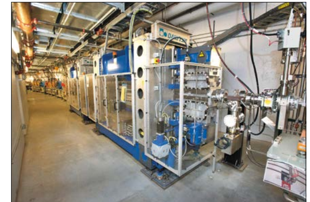
One of six damping wigglers, used to reduce beam emittance.
