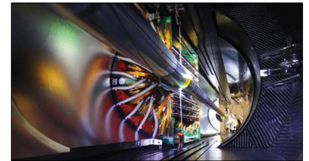
Fig. 3. The barrel pixel tracker being re-installed around the beampipe, December 2014.
