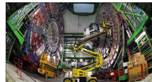
Fig. 2. CMS ready to close, showing the beampipe and the extensive new environmental seal.
