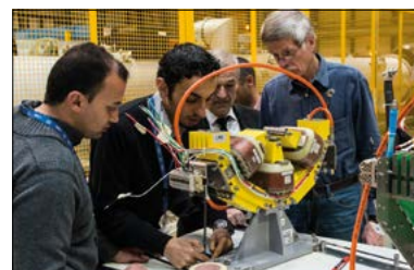
Top: The first cell for SESAME, assembled and tested at CERN, with one bending magnet (red), two sets of focusing and defocusing quadrupoles (green) and four sets of correcting sextupoles (yellow). (Image credit: CERN-PHOTO-201503-059-57.) Above: Experts from CERN and SESAME with part of a sextupole assembly. (Image credit: CERN-PHOTO-201503-059-9.)
