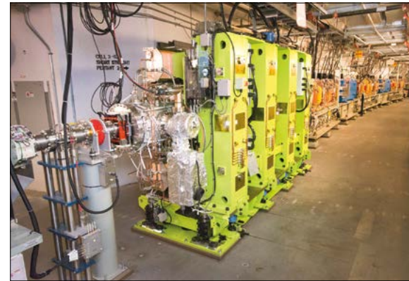
One of the four in-vacuum undulators – the workhorses of NSLS-II.
